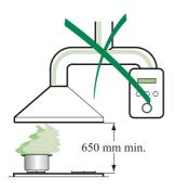
Check that the mains voltage corresponds to that indicated on the rating plate fixed to the inside of the hood.
